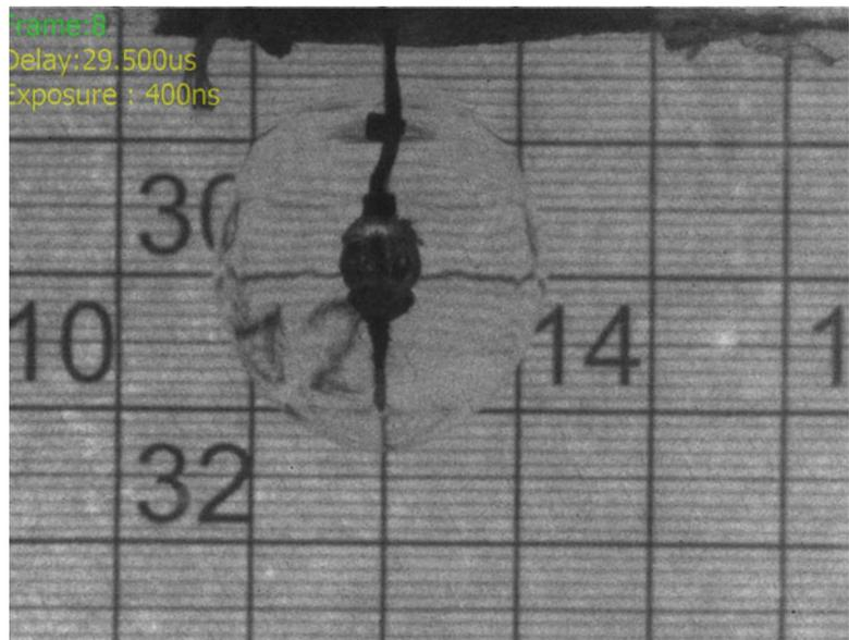
**Fig. 11.5** Underwater RP-1 detonator during ideal detonation
