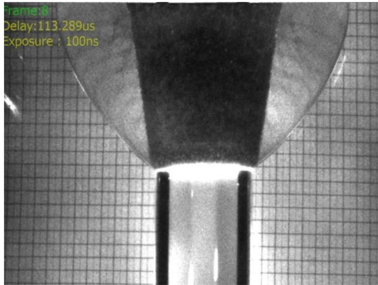
**Fig. 11.2** Velocity of detonation for the reaction front
