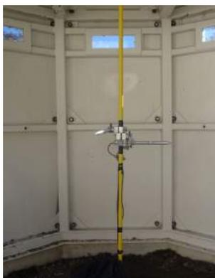
A pressure gage is placed inside AXPRO's blast chamber.
